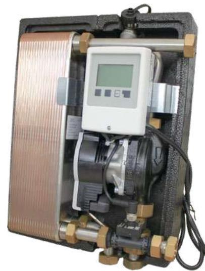
**Application:** The eco 25 fresh water station is ideal for the central heating of drinking water in heating systems. The heating water is taken from the buffer tank and passed through the plate heat exchanger to heat the drinking water directly as required. A buffer tank is required to ensure the necessary heating water flow rate.
