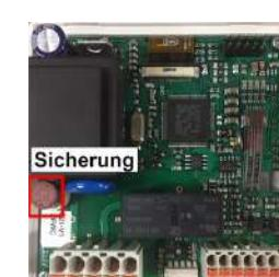
If the controller does not function and there is no display despite the mains voltage being switched on, the internal device fuse may be defective. In this case, open the device as described in 3.2, remove the old fuse, and check it.
