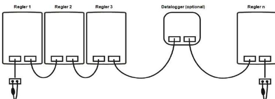
1. The controllers are connected in series using the CAN bus cable.
