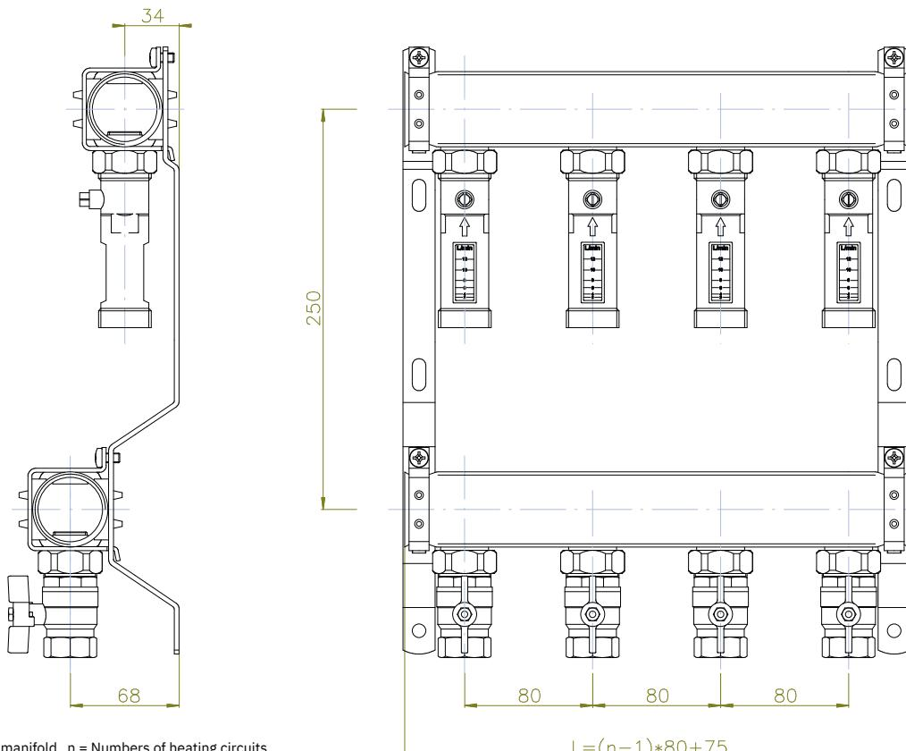
L = Length of the manifold n = Numbers of heating circuits
