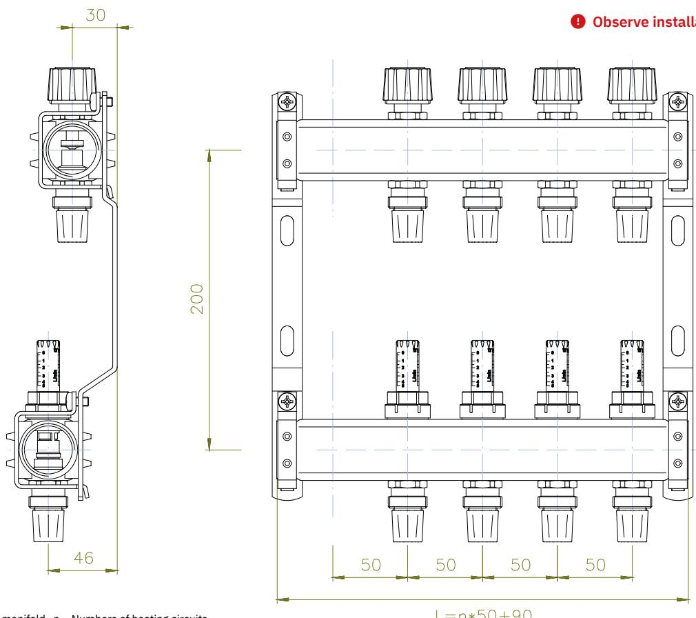
L = Length of the manifold n = Numbers of heating circuits
