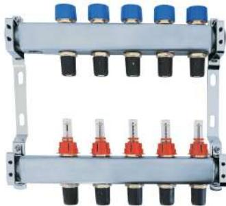
**Items delivered:** Set consists of supply and return bar, each with two G½" internal threads for vent valves. Pre-assembled in sound-insulated holders, including labelling stickers and adjustment instructions, packed in cardboard box.
