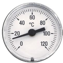
The thermometers are specially designed for ball valves with an integrated thermometer holder. They enable reliable and direct temperature measurement in the heating or drinking water system. Thanks to the simple plug-in installation, they can be inserted without tools and easily removed if required.
