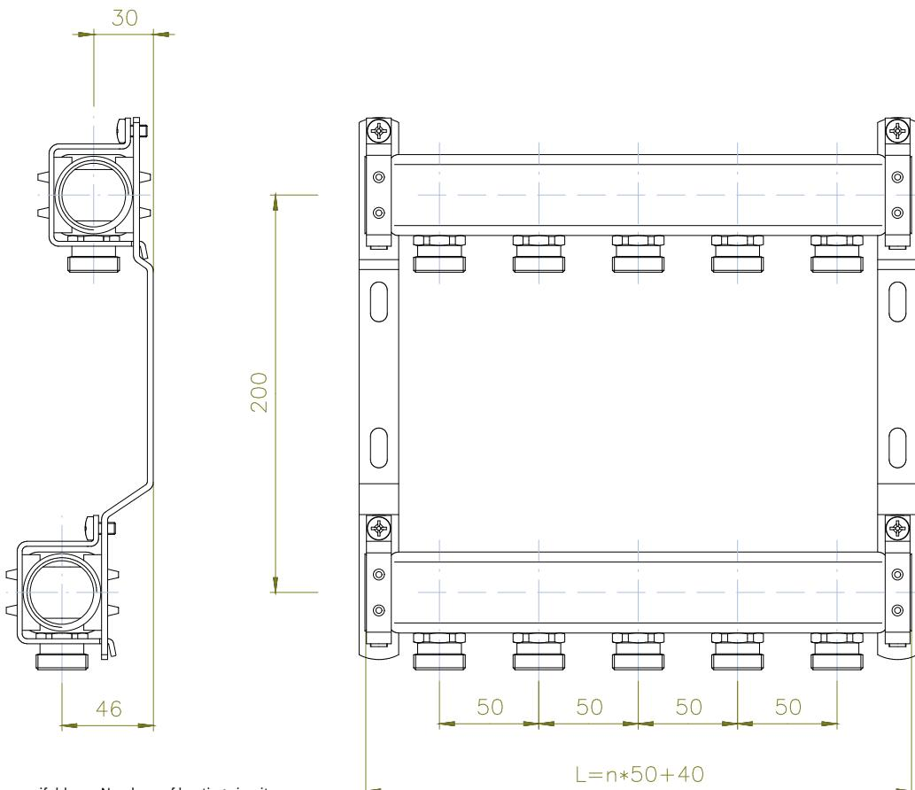
L = Length of the manifold n = Numbers of heating circuits
